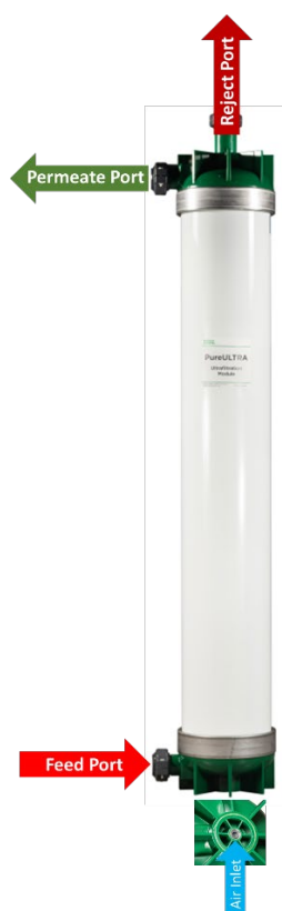
Figure 5. PureULTRA II Module Structure
