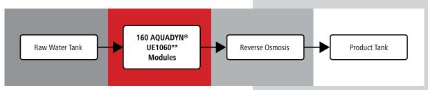
This project involved a variety of challenges, however, the main goal was to provide a more compact system with a lot smaller footprint than the previous treatment system. The existing system included a flocculation, a settler and a filtration step. Additionally, the new treatment plant needs to absorb possible variations in the raw water composition while delivering constant effluent quality.
